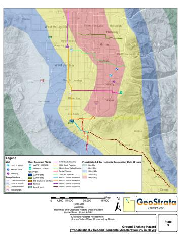
The Jordan Aqueduct has multiple segments that pass through ground acceleration zones. A large earthquake could damage and seperate the pipeline.
