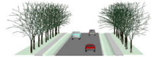
Above: 24 foot pavement with curb and swale in a 66 foot Right-of-Way, adapted from the Two-Lane Cross Section, Figure 4-1 in the Perry City Transportation Master Plan. Below: 39 foot pavement with curb and gutter (42 feet from curb to curb in a 66 foot Right-of-Way).
