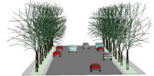
Above: 24 foot pavement with curb and swale in a 66 foot Right-of-Way, adapted from the Two-Lane Cross Section, Figure 4-1 in the Perry City Transportation Master Plan. Below: 39 foot pavement with curb and gutter (42 feet from curb to curb in a 66 foot Right-of-Way).
